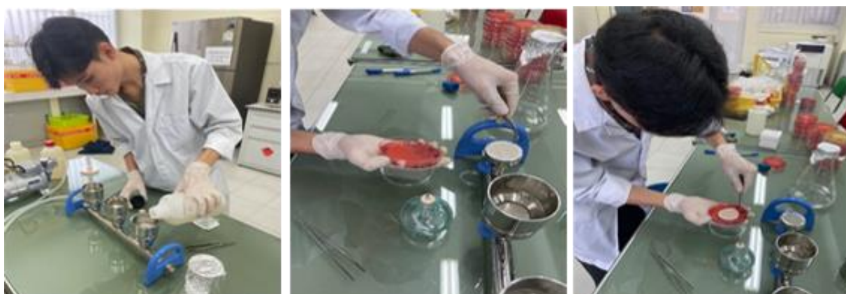
Figure 3.3. Procedure for microbial culture by using filtration method
