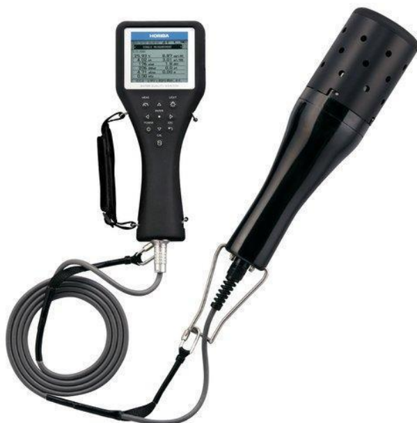
Figure 3.2. Horiba U-50 multi-parameter water quality checker
