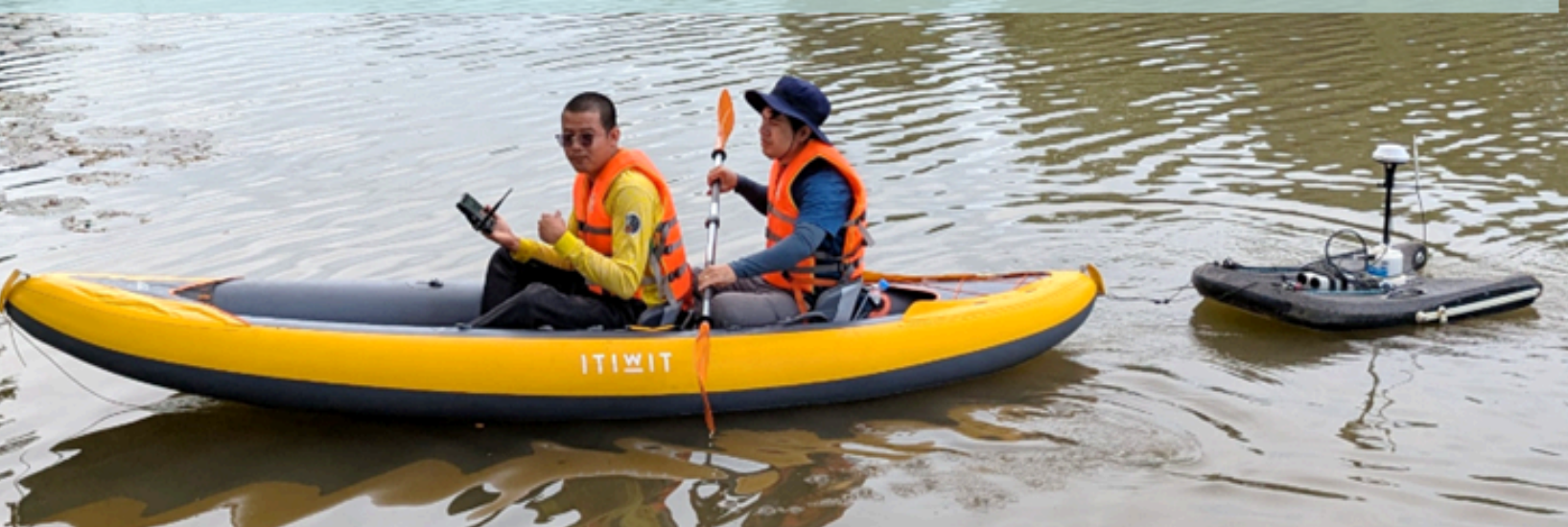
Mapping the depths: A bathymetric survey underway in the Banteay Chhmar temple moat using an Acoustic Doppler Current Profiler mounted on a small boat towed behind (28 October 2025)
